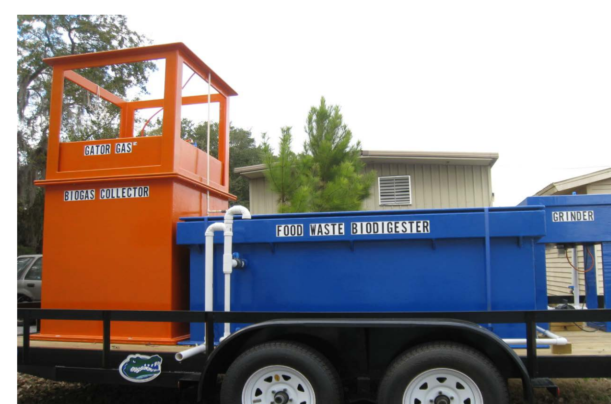
Figure 2: Portable food waste digester for demonstration at schools and restaurants
